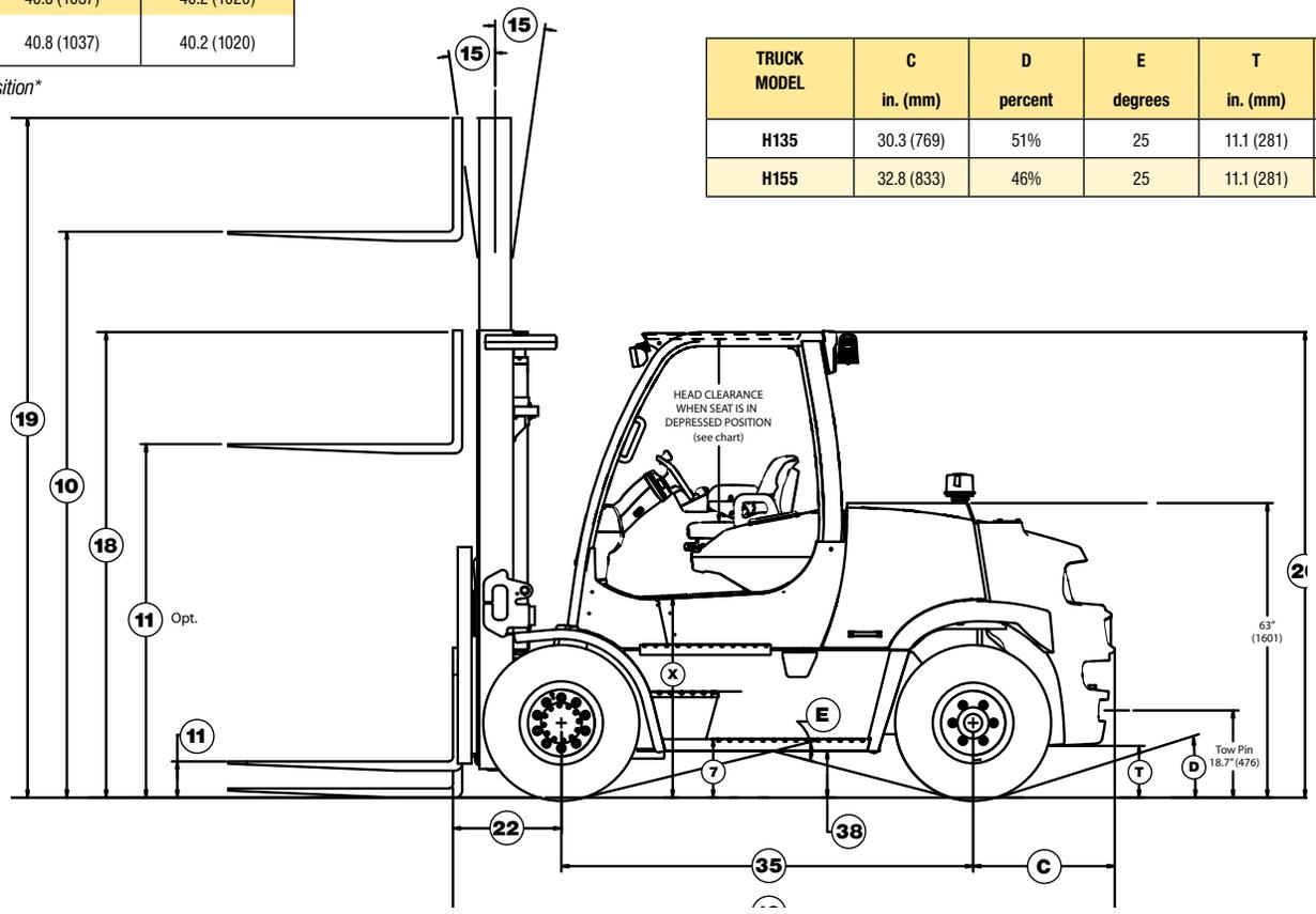
Circled dimensions correspond to the line numbers on the tabulated chart inside the Technical Guide. Dimensions are in inches (millimeters).
