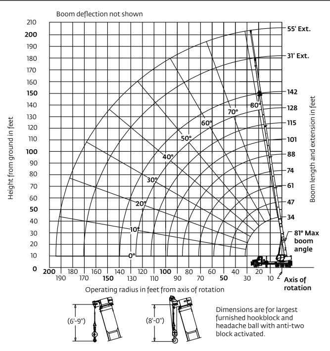
\*Drawing is to show the physical reach of the machine. Always refer to load chart to see what portions of this range are structurally and stability limited.
