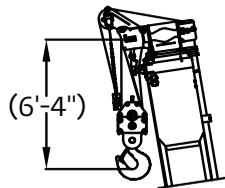
Dimensions are for largest furnished hookblock and headache ball with anti-two block activated.
