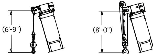
Dimensions are for largest furnished hookblock and headache ball with anti-two block activated.
