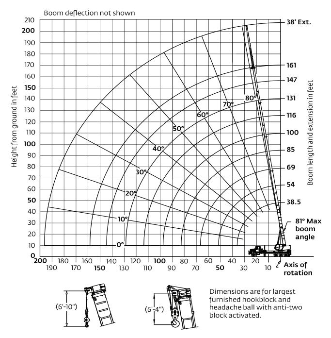
\*Drawing is to show the physical reach of the machine. Always refer to load chart to see what portions of this range are structurally and stability limited.
